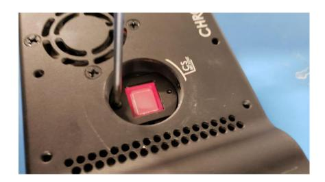
3. Using tweezers, very, very carefully push the IR filter up so you can grab one end. When grabbing it with tweezers, it **will** scratch it, only touch the part where the lens rests on the frame, not where the sensor looks through.
