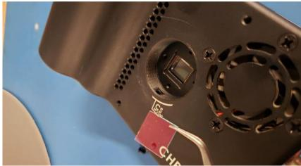
4. The IR filter is now removed! Reverse these steps to reinstall it.
